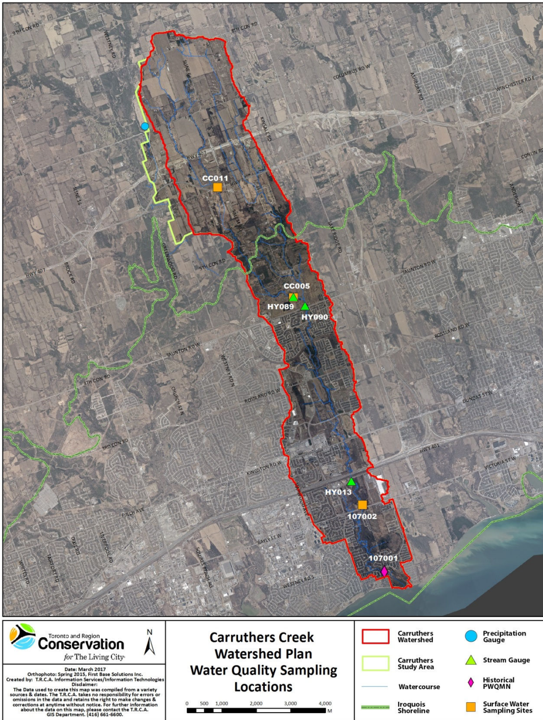
Figure 2. Study area for Carruthers Creek watershed plan with sampling locations (CC011, CC005, 107002), and local precipitation (HY015) and stream (HY089, HY090, and HY013) gauges.
